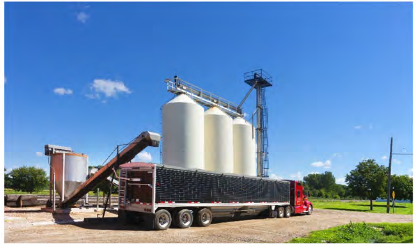
A sixth axle significantly reduces the burden on infrastructure
